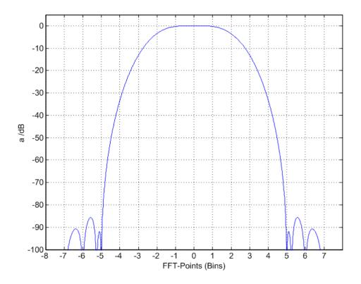
Figure 5: Flat-topped frequency spectrum window. The noise bandwidth is 3.86/(measuring time) = 3.86/400 ms = 9.75 Hz in the default state, which is equivalent to 3.88 bins.
