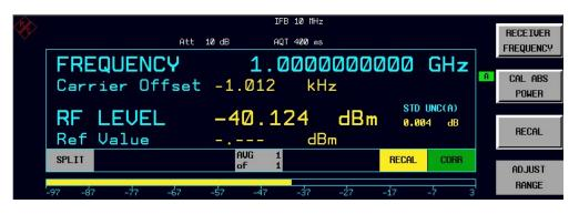
Figure 1: A portion of the FSMR display with the recalibration prompt (**RECAL**).
