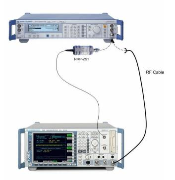
Figure 6: Using an NRP-Z51 power sensor as a reference sensor for high absolute level measurement accuracy with the FSMR
