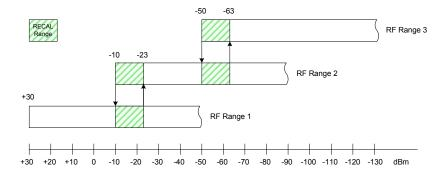
Figure 3: Graphic representation of the FSMR power level ranges
